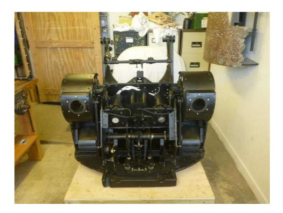
The view from the rear shows the oxygen pipe heading off towards the economiser which is now located in the top rear of the cupola, behind the gunner's head. Also visible is the later standard of seat which allows the gunner to sit on a 'pilot's type' parachute. This seems like a very good idea as it removes the need to reach into the aircraft to retrieve your parachute before bailing out. This modification also moves the Gyro Gun Sight (GGS) junction box to just in front of the seat.
